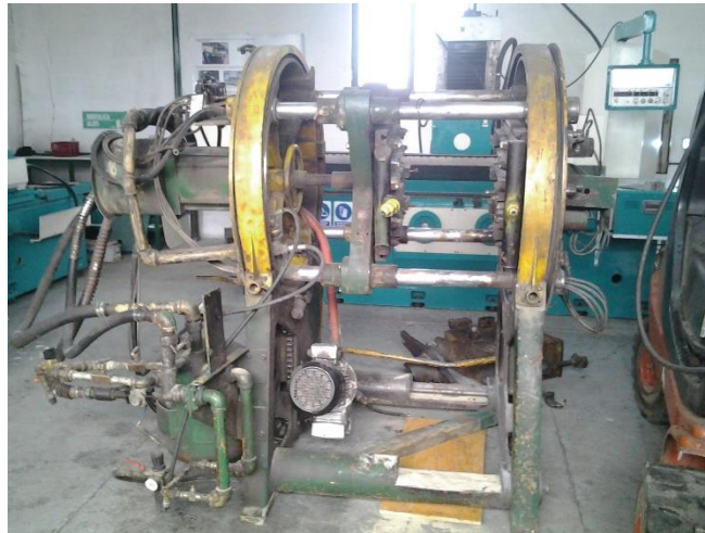
Fig. 2. Machine after dismantling the electrical installation [9]
