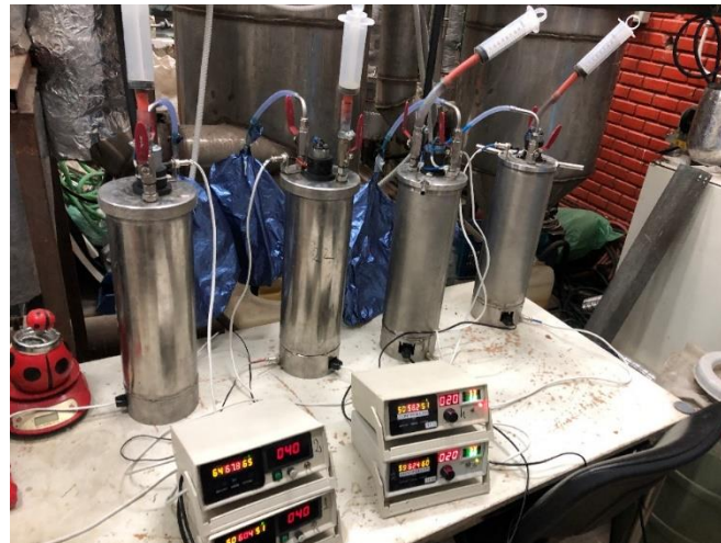
Figure 2 – Standard inox reactor
