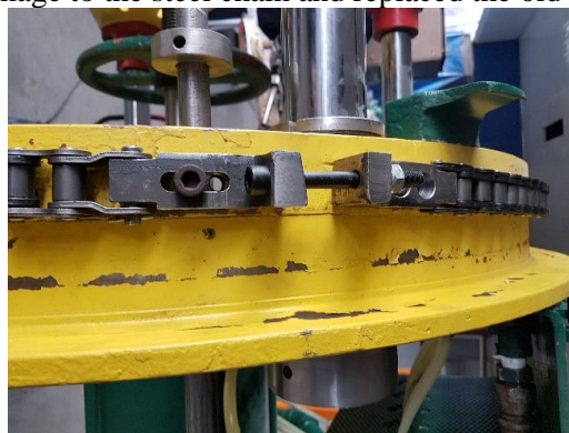
Fig 6. Replaced steel chain [9]
