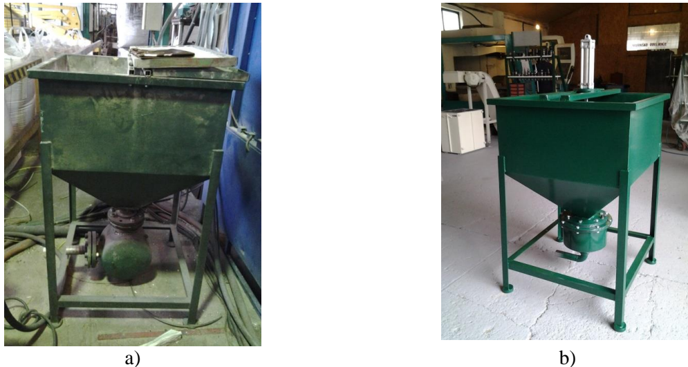
Fig. 5. Additional reservoir for sand a) before and b) after reparation [9]
