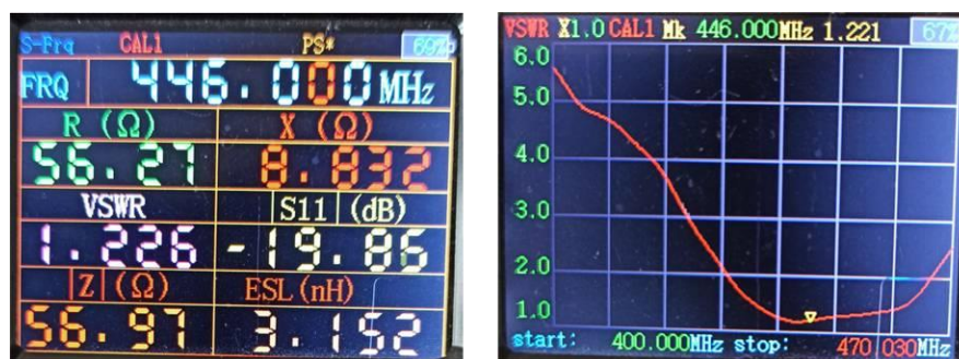
Fig. 9. Common electrical parameters of a two stacked Quad antennas and VSWR vs frequency of a two stacked Quad antennas, each with four elements.
