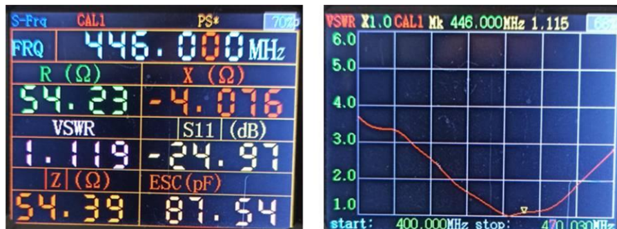
Fig. 8. Common electrical parameters of a two stacked Quad antennas and VSWR vs frequency of a two stacked Quad antennas, each with three elements.
